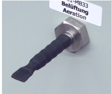
Fig. 6: Hose nozzle of the aeration valve with heat shrink tube
