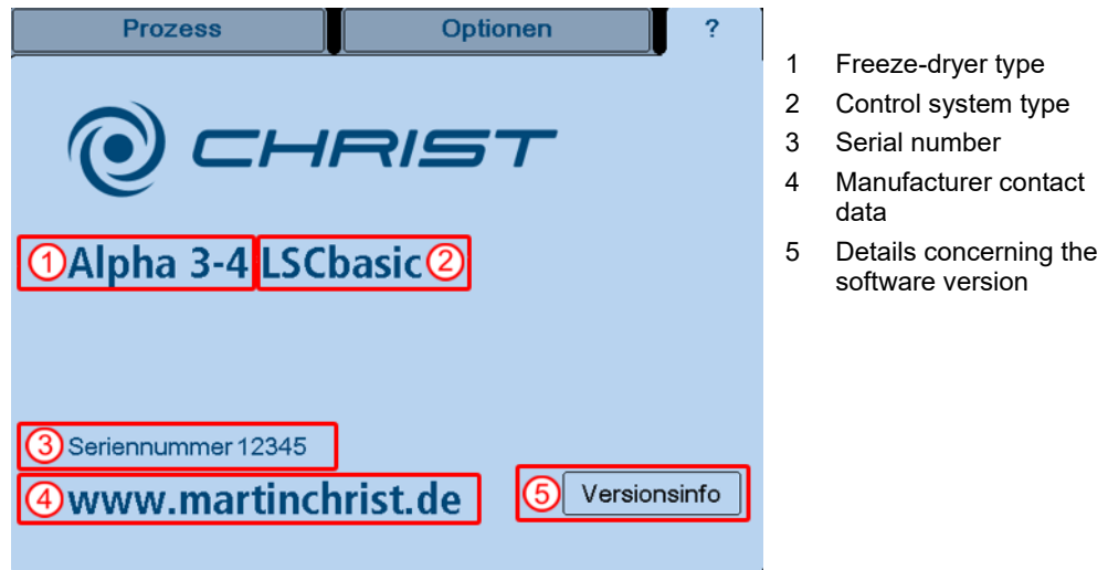
Fig. 52: Freeze-dryer system information, here for Alpha 2-4 LSCplus
