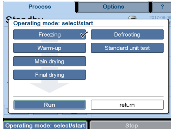
Fig. 33: Dialogue box "Operating mode: select/start" (The version of the dialogue box that is displayed depends on the equipment of the freeze-dryer.)
